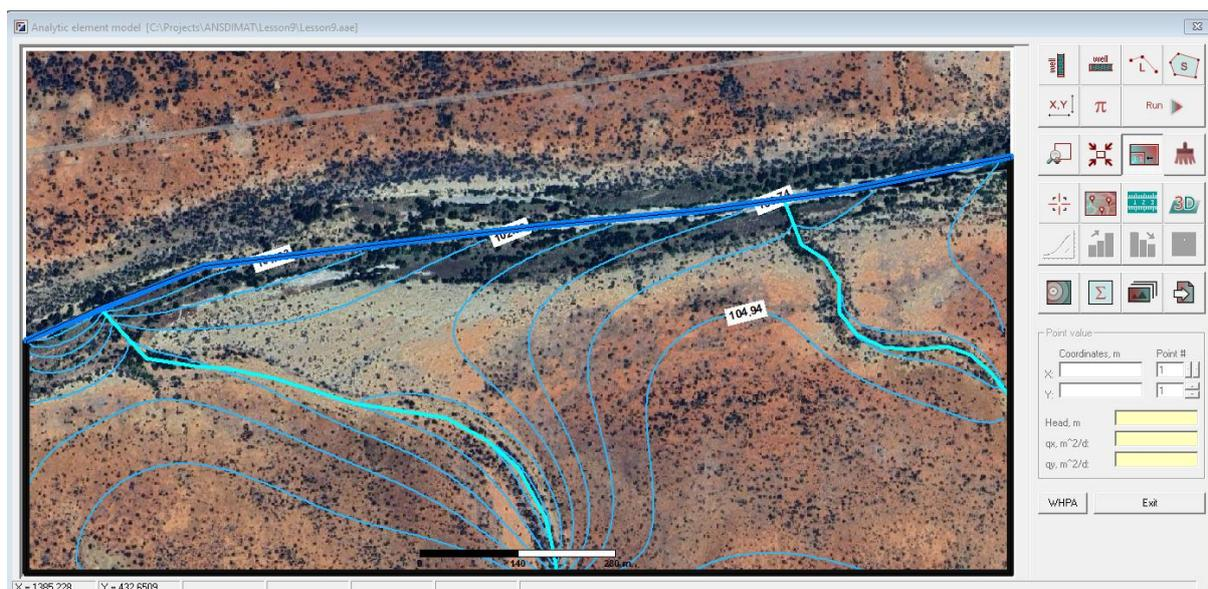
**Figure 19:** Contours showing the piezometric heads calculated for the model area without the excavation.
