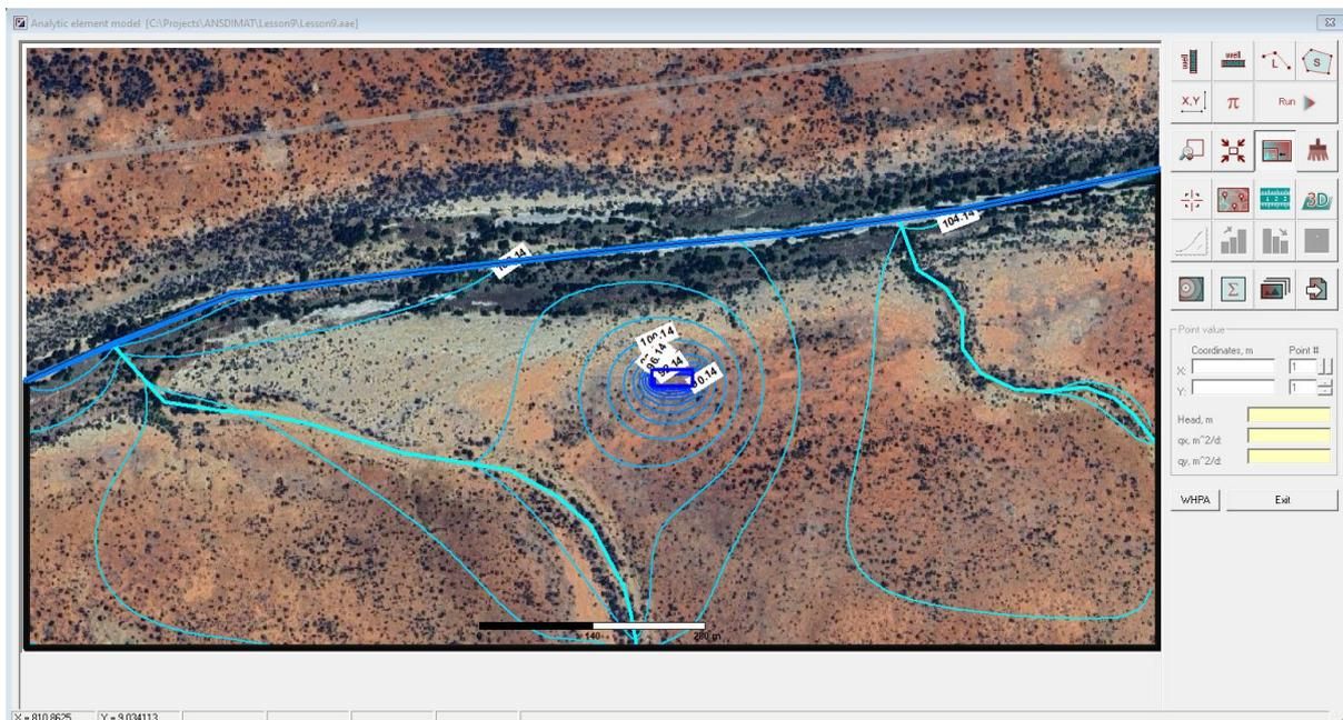
**Figure 21:** Contours showing the piezometric heads calculated for the model area including the excavation and the barrier stopping the water inflow from the main river.
