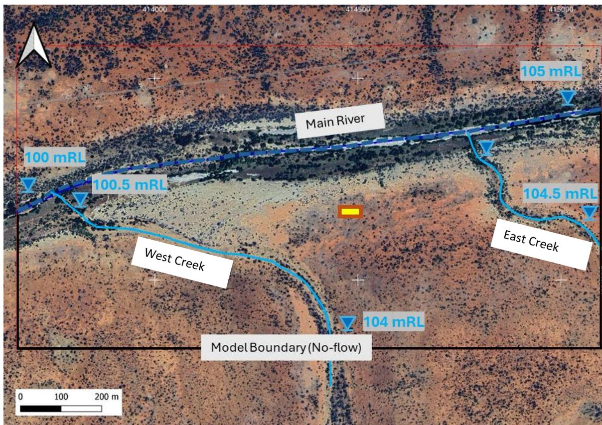
**Figure 1:** Location map showing the excavation (yellow) and the barrier (brown, one of the modelled options); the dark blue striped line indicates Main River (time-constant head boundary); the light blue lines – West Creek and East Creek (transfer boundary condition or “river-boundary in ANSDIMAT”); the black lines show the outer model no-flow boundary; the thin red line marks the limit of the project map; numbers on the map refer to water levels in the main river and tributaries.
