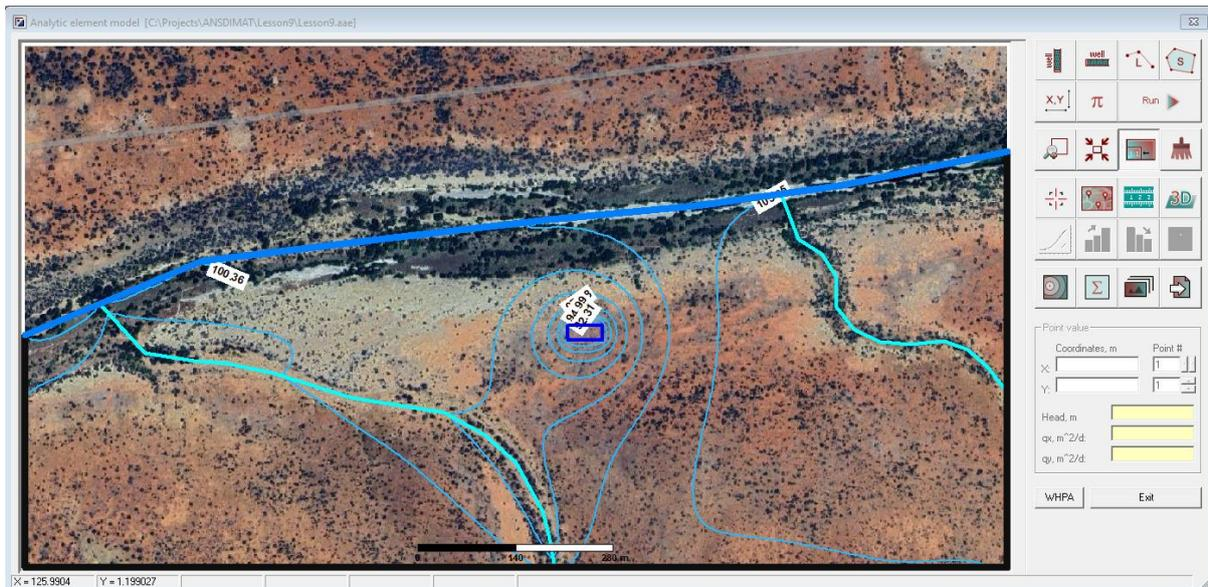
**Figure 20:** Contours showing the piezometric heads calculated for the model area including the excavation.
