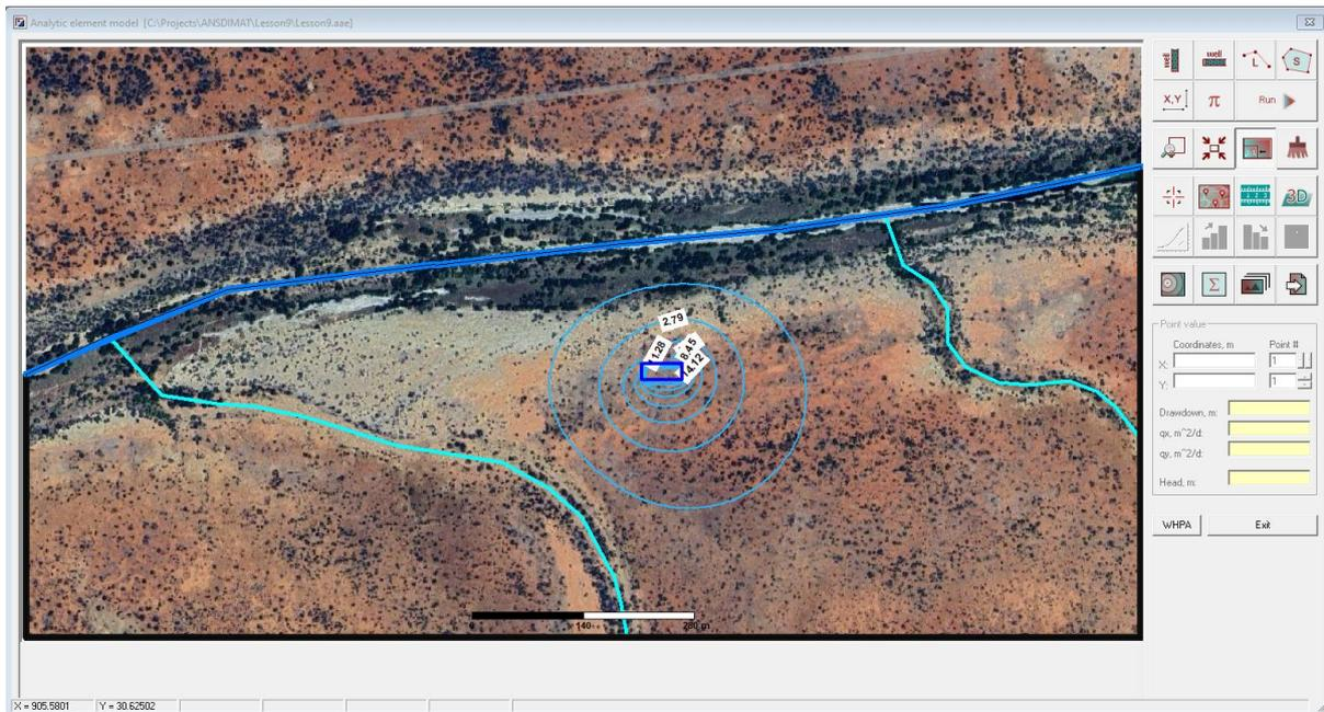
Figure 25: Contours showing the drawdown calculated with initial heads set without the excavation and the current model including the excavation and the barrier.
